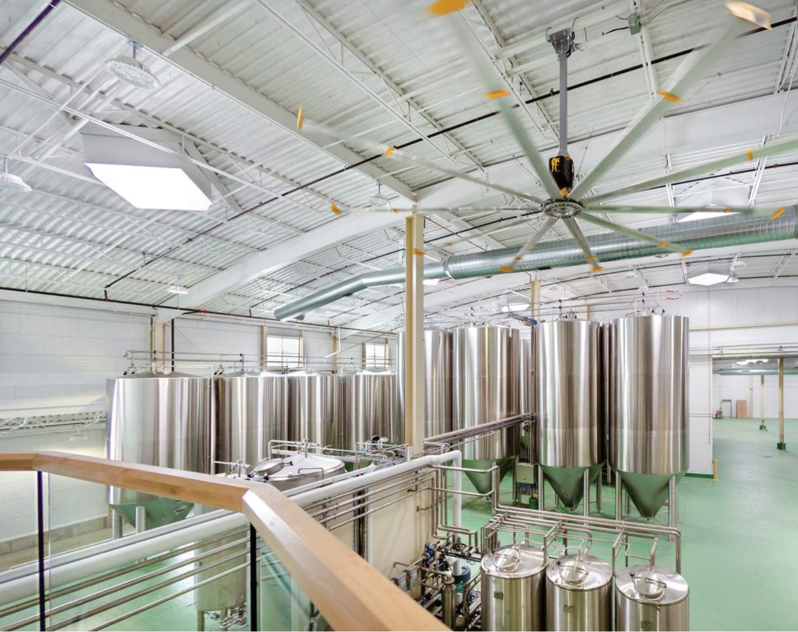
The view from the mezzanine of the main brewery floor of the 35,000 sq. ft. von Trapp Brewery and Bierhall in Stowe. When the brewery equipment arrived from Europe, it was lowered via crane through the roof opening and rigged into place by Neagley & Chase crews. Stina Booth photos.
